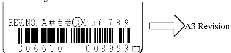
Figure 1.2 Display of disk drive revision number
